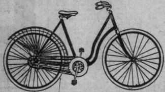
Frame is 22 and 24 inch, of nickel steel 1 1/2 inch tubing...
