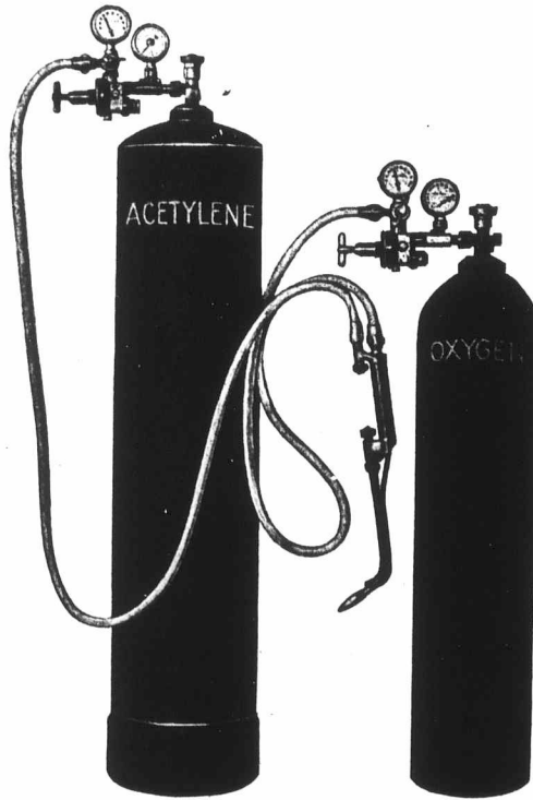
Welding Plant Ready to Operate.
