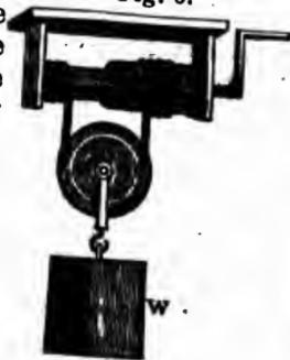
88. For the differential wheel and axle let  $d$  = the difference between the radii of the axles,  $R$  = radius of the wheel,  $P$  = the power, and  $W$  = the weight.
