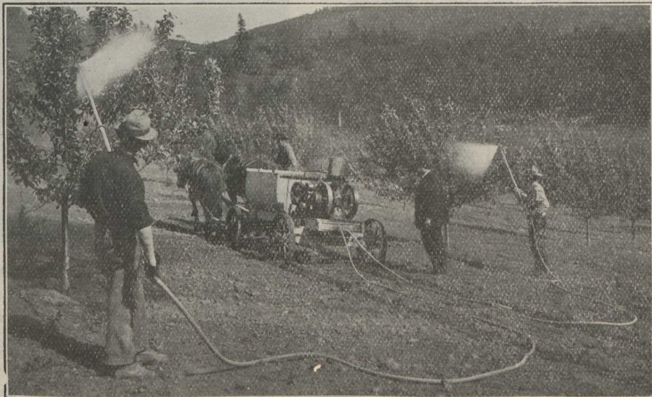
A Modern (Hardie) Power Sprayer at Work in a Western Orchard—Note the Advantage of Low Trees
