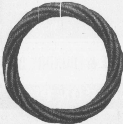
Appearance of Durable Wire Rope after three months use, night and day, for transmission of power
