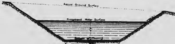
CROSS SECTION OF UNLINED OPEN CHANNEL
