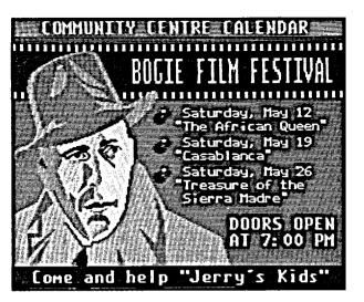
These pieces of text, with codes indicating their priority and the chosen graphic, are run into a minicomputer dedicated to the Infovision service. Software in the Infovision computer fetches the chosen graphic from its library of graphics, puts it together with the text, and then checks the new item's priority.
