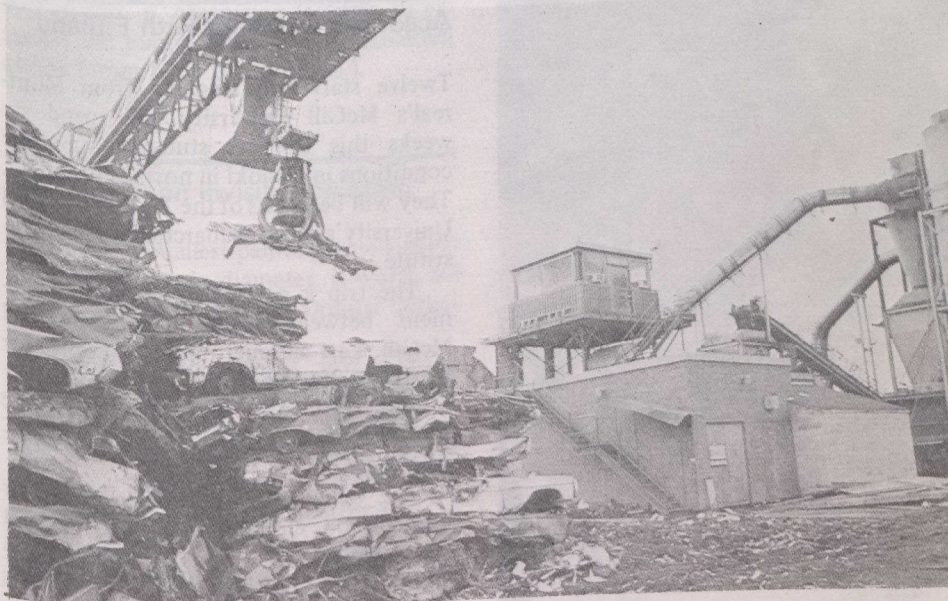
Powerful claws pick up a junked car and lift it to the mouth of a car shredder. On the right is the pneumatic sorter, which removes light debris from shredded car material.
