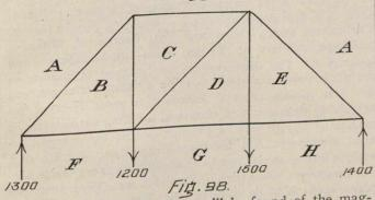
plied, the abutment reactions will be found of the magnitudes indicated on the diagram.
