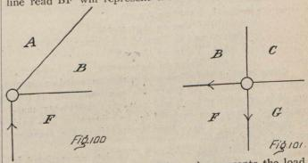
point BFGC. The line FG (Fig. 99) represents the load FG. (The load FG is less than the reaction AF.) The lines GC and CB complete the polygon, which should then read: BF, FG, GC, and CB. The members GC and CB are evidently both in tension.
