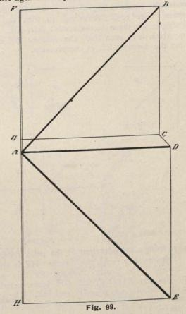
in tension and the member BA in compression. (The magnitudes of these stresses will, of course, be given by scaling the lengths of the lines FB and B.A.
