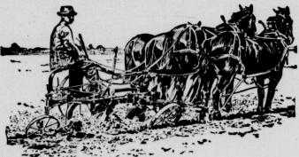
LIVER plows have many strong points of superiority. The tractor gangs are made up of 4, 5, and 6-base sections. With these sections you can build up a gang with any desired number of bases. The sections are joined together flexibly so that an Oliver follows the lay of the land and plows to an even depth. The small sections are easily handled and require little room for storage.
