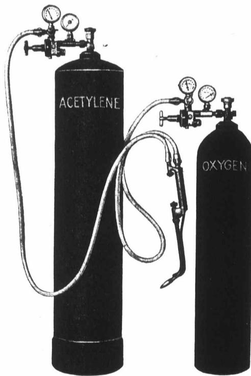
Welding Plant Ready to Operate.
