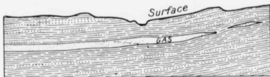
Fig. 33. Section through strata, showing example of gas accumulation in the upper portion of a sand stratum which plays out.
