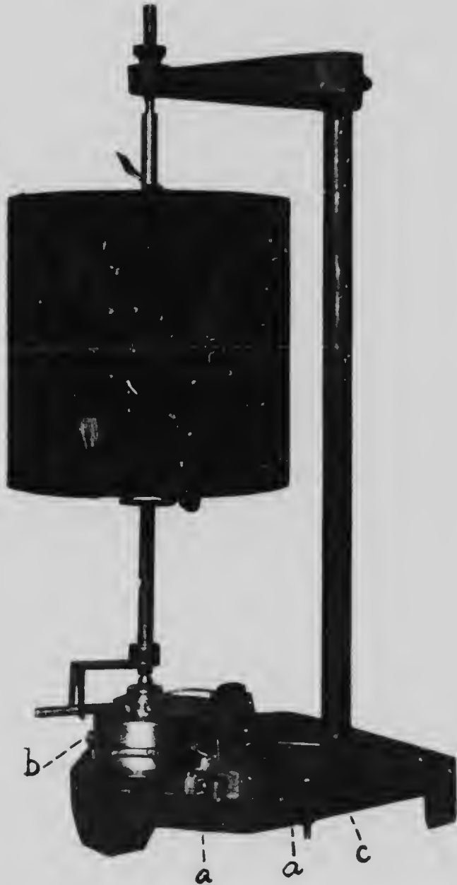
FIG. 5. Rapid kymograph. (a) Terminals to be connected in primary circuit; (b) Movable ring for second stimulus; (c) Release which starts drum.
