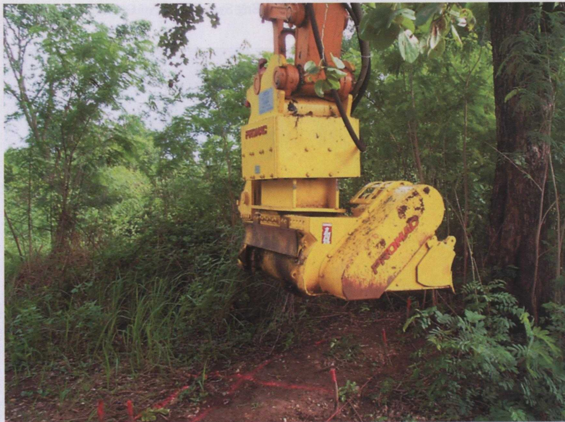
Adapted for mine clearance operations with an investment from Technology Partnerships Canada, the PRO MAC Brushcutter/Deminer BDM 48 undergoes trials in Thailand.
