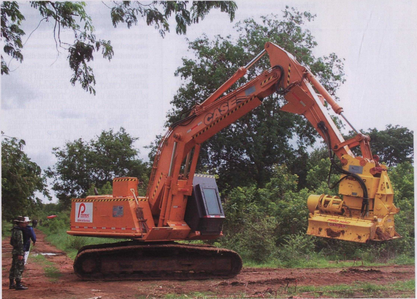
Adapted for mine clearance operations with an investment from Technology Partnerships Canada, the PRO MAC Brushcutter/Deminer BDM 48 undergoes trials in Thailand.
