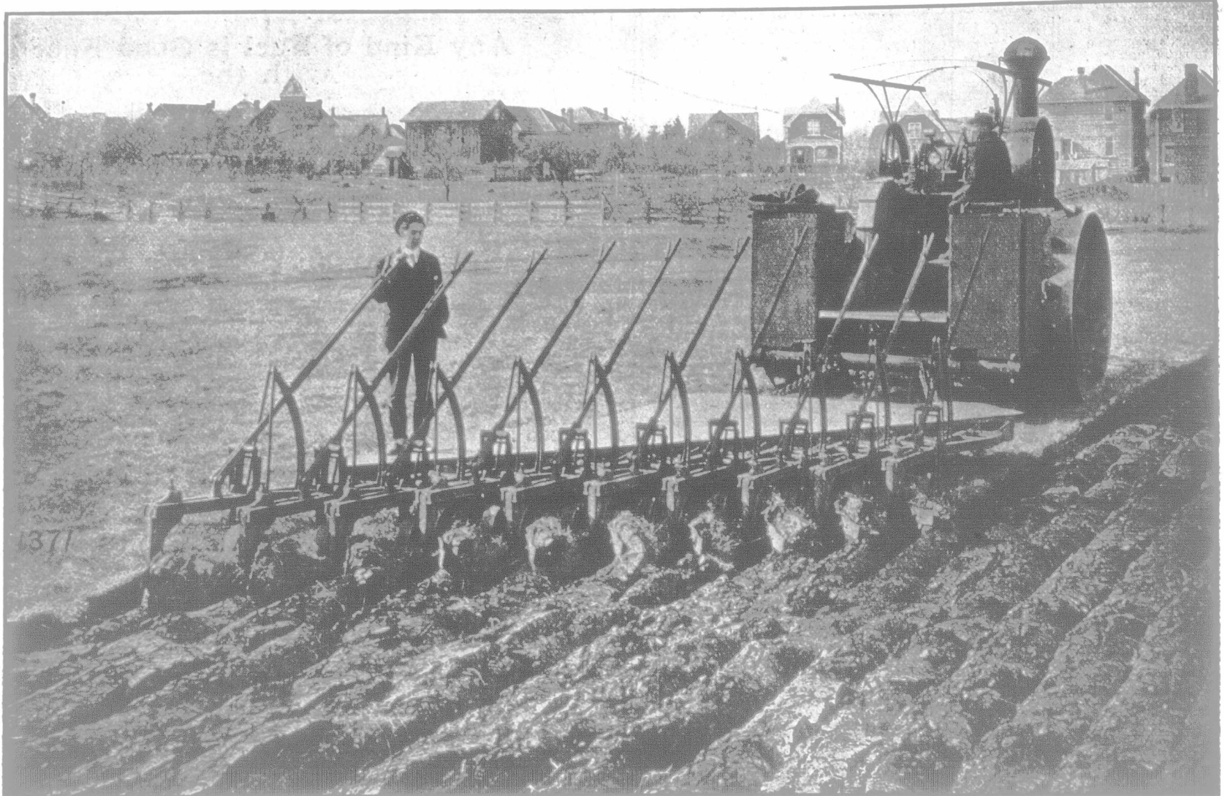
Waterous New Plowing Engine with Waterous Improved Plow Hitch The Latest and Best Design of Plow Hitch in the Market
