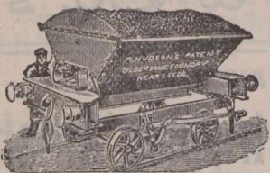
59—R. H.'s Patent 6-Ton Steel Double Side Tip Wagon, to work with ordinary 10 1/2 Wagons
