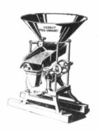
THE Vessot "Champion" cleans grain as well as grinds it. The spout that carries the grain to the grinder is made with two sieves, a coarse one above and a fine one below. The coarse sieve catches nails, sticks, and stones, but lets the grain fall through. The fine sieve holds the grain, but takes out all sand and dirt. The grain passes to the grinding plates as clean as grain can be.
