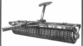
The Western Pulverizer, Packer and Mulcher pulverizes and packs down the soil and puts it in perfect condition for seeding in one operation, either a stubble ground or sod ground. It will not clog. Provides a granular mulch to the land which stops evaporation and preserves moisture.
