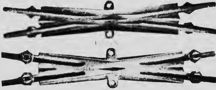
FIG. 1478. 15° Fixed Crossing, Frog, as Seen from Above.
