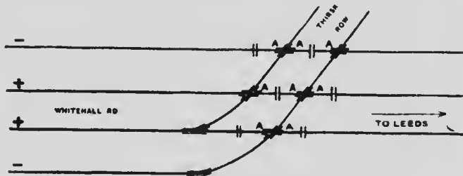
Fig. 1,528. Diagram of Insulation Arrangements at a Junction.
