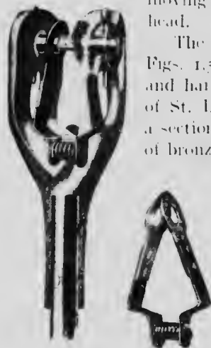
Fig. 1, 10. Trolley Harp showing Details of Rubbing Contact.
