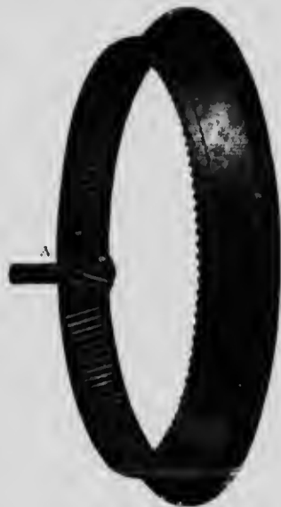
Fig. 1,605.—Helically-cut Transmission Gear.
