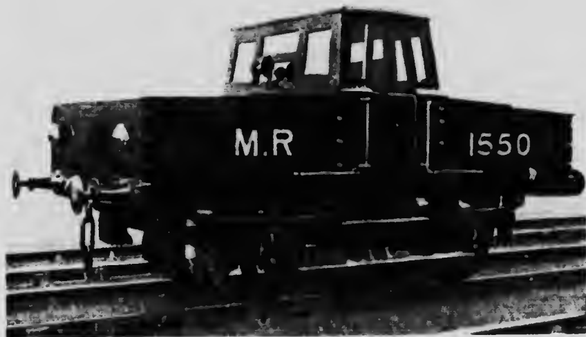
Fig. 1,805.—A battery-driven Shunting Locomotive.
