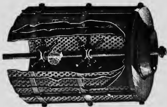
Fig. 6 (b). Concentric cylindrical trommel.
