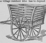
A HOMEMADE HAND CART. elbarrow, or some such arrange as this to move his small crops and other stores. The sides and ends fit tightly into iron sockets, and, for stability, lock to-gether at the corners when in place, as shown in the engraving. Any one handy with tools can construct a very serviceable rig of this sort, the only necessary adjuncts being a pair of wheels, which are often at hand, from some broken or worn-out wagon, sulky, or other light vehicle.—Amorican Arginaltunic
