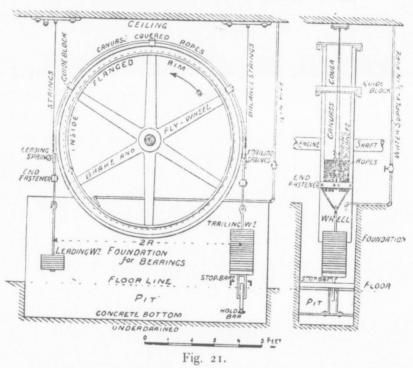
This brake, which was designed to determine the work done by a fifty horse power experimental engine, has given such satisfactory results in use,
