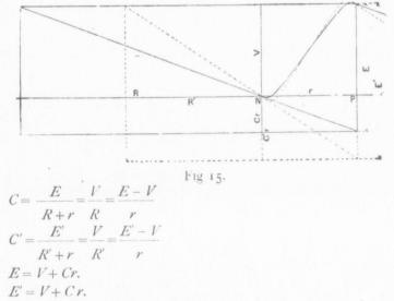
The electromotive force E, generated by the dynamo, is seen by referring to the graphical representation to be the sum of the difference of potential between the brushes V and the product of the current flowing and the internal resistance of the armature Cr. E = V + Cr. The greater the current, the greater must E be to maintain V constant.
