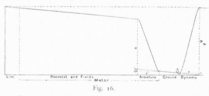
$E = \text{generated } EMF \ e = \text{counter } EMF. \ E - e = \text{effective } EMF.$  $C = \frac{E \cdot e}{R}$ , where R is the total resistance of the circuit.
