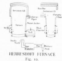
The furnace is provided with a well or receiver, into which the ore runs as it melts in the furnace. This receiver is a cast-iron water-jacketed chamber, lined throughout with fire brick set in fire-clay cement. It has
