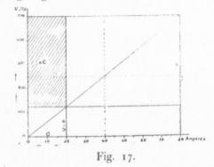
Horizontal distances represent currents, and vertical ones differences of pressure. The hatched area represents the work done by the motor, and this is a maximum when  $e = \frac{V}{2}$ , as is readily understood. The efficiency is  $\frac{e}{V}$ .
