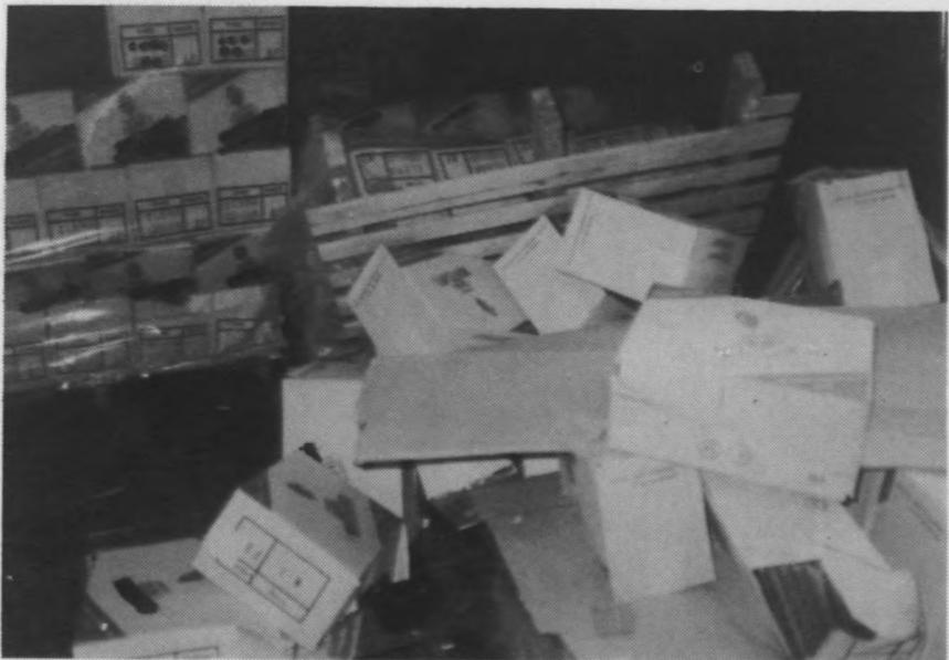
*No cargo separations, no proper layering or bracing.*
