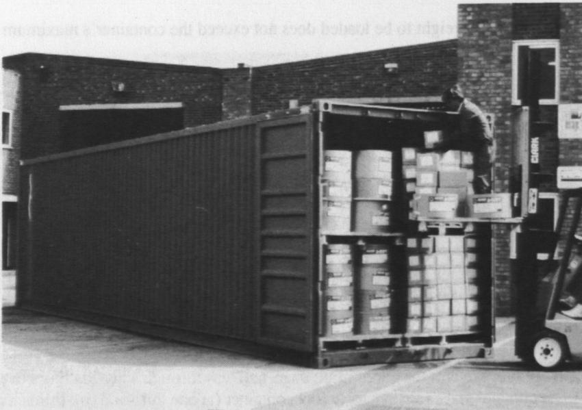
*It looks good, but it will probably be delivered in a damaged condition because of improper stacking, no cargo separation, no proper layering or bracing.*
