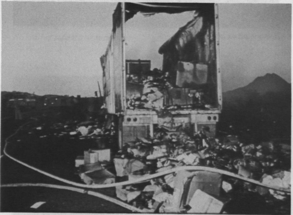
*Explosion from friction by loose cargo*
