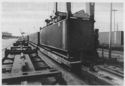
Overhead crane discharging container from rail car.
