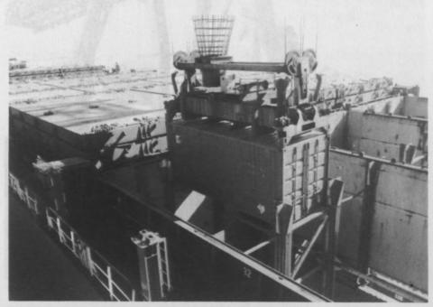
Container crane loading container into cellular containership.
