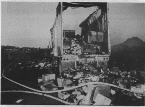
Explosion from friction by loose cargo
