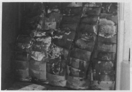
Too tight a stow, no separations, container leaked causing water damage.
