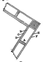
Fig. 2. (A) Studs. (B) Inch lumber. (C) Tar paper. (D) Matched or planed lumber. (E) Tar paper. (F) Outside siding. (J) Post.
