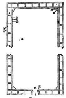
Fig. 4. (A) Studs. (B) Inch lumber. (C) Tar paper. (D) Matched or planed lumber. (E) Tar paper. (F) Outside siding. (G) Door. (H) Cleats. (I) Outside door on hinges, and in two or three pieces. (N) Corner board. (O) Sawdust.
