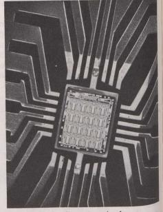
Integrated circuit on a carrier frame.
