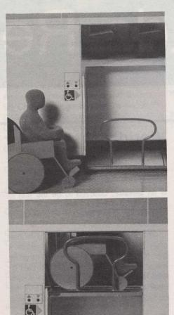
Design concepts from Rutenberg Design Inc. show how a passenger is transported some 100 centimetres inside the bus from the curb to seating level.
