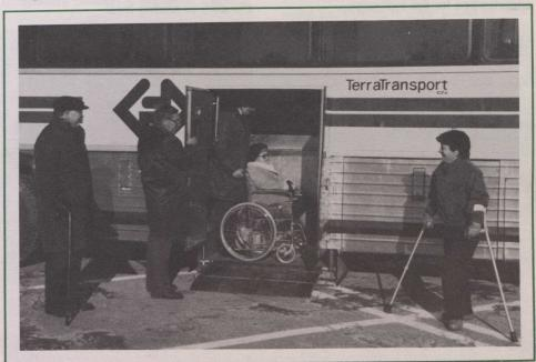
Inside elevator on intercity bus allows easy access for disabled passengers.
