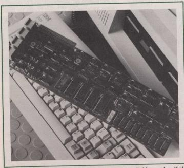
TIL Systems' XPERT PC Card provides packet switching and multiple terminal emulations for any IBM-compatible personal computer.
