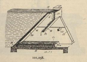
a grating covering the same. The heel wall extends downwardly and inwardly below said opening in said deck so that the water flowing through will strike said inward incline and be directed backward and fall on a wear resisting bed from where it flows on down stream. Tube Cleaner.—Thomas Andrews.—101,594.—The above invention is a novel form of tube cleaner in which steam is injected through the instrument into the tube. The steam
