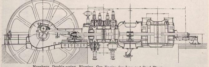
Nurnberg Double-acting Blowing Gas Engine for Iron and Steel Plants.
