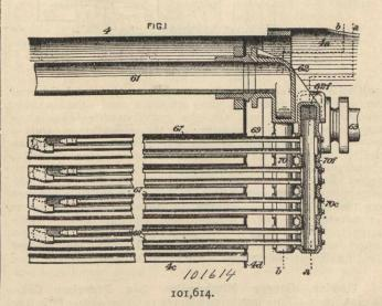
tubes, a superheated steam header separate from said saturated steam header connected to the forward end of the other pairs of superheater pipes. A T-head connection having a communicating passage from the supply compartment in communication with the saturated steam header to the delivery compartment from the superheaded steam header and a wall partially interposed between said chambers.
