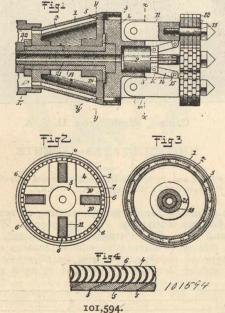
in passage through the instrument is directed through a number of ports against the buckets of a turbine wheel and a rotor scraping tool is secured to and rotated by said turbine.
