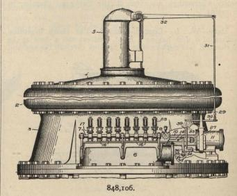
It consists of mechanically-operated nozzle-valves, of a liquid-pressure motor for operating them, means for causing of annular groups of pockets, each pocket having an impact inner side, each pocket opening its whole length into the side of the runner, the inner side being concentric to the resistance to movement, and an air-chamber.
