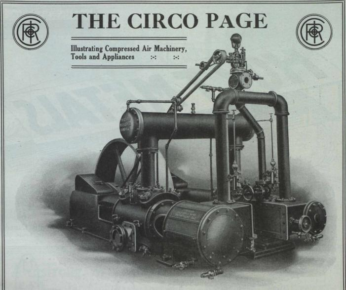
Class "RL-3" Duplex Type, Steam Driven Air Compressor, with Cross Compound Steam and Cross Compound Air Cylinders with Intercooler. Machine is convertible to Belt Drive when required, and is equipped with Speed and Pressure Governor, "Circo" Silent Leaf Inlet and Outlet Valves, Enclosed Dust-Proof Construction, Splash Lubrication System and Meyer Adjustable Cut-off.
