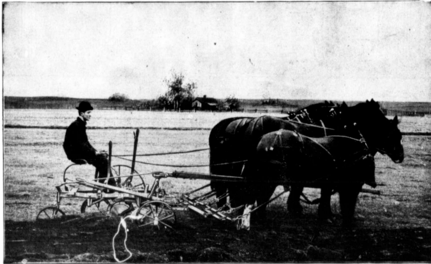
Oliver No. 1 Gang. Four horses hitched abreast, but none walking on the plowed ground.
