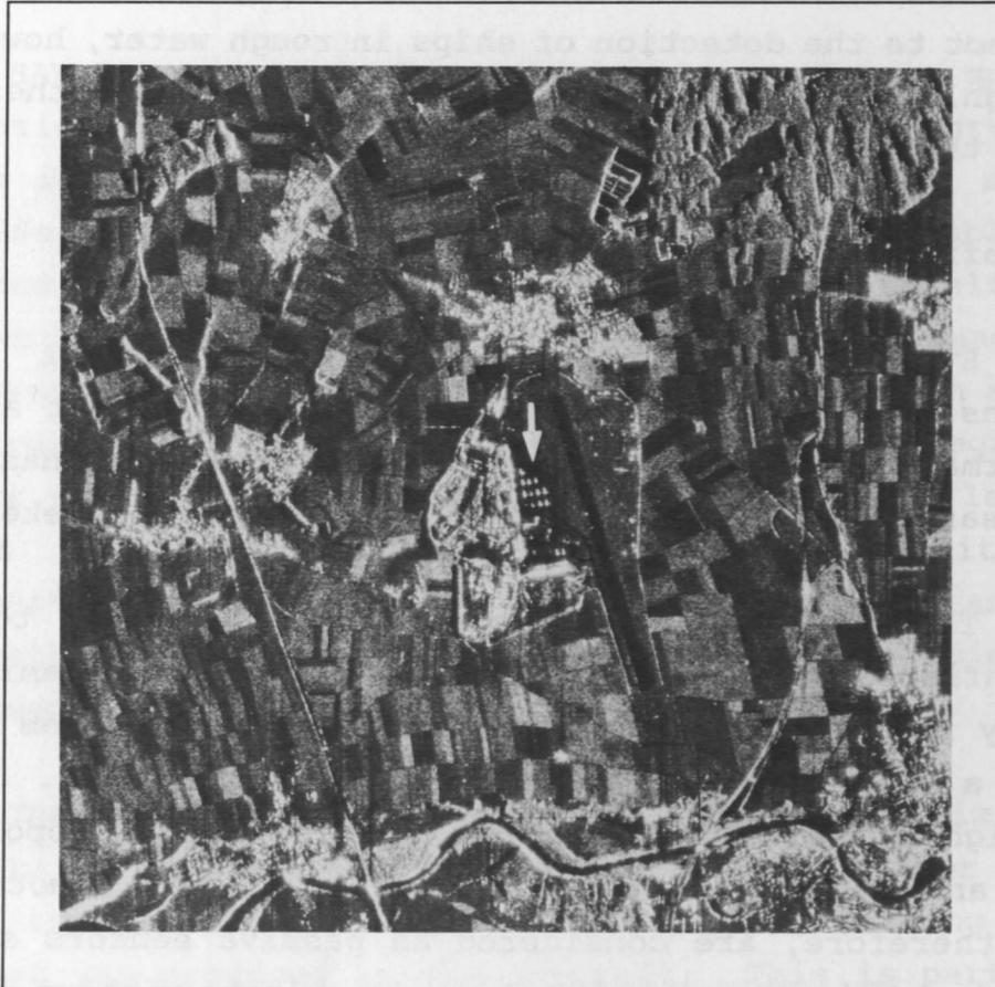
This SAR image was acquired over an airfield from an altitude of 10,000 m above the ground. Note the aircraft on the apron and their relative position near the runway. The length of runways and airstrips can be readily measured using this type of airborne imagery. (Image courtesy Intera Technologies Ltd.)
