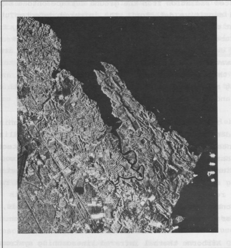
The bright targets on the right side of this SAR image are "mothballed" ships docked in a bay. Note the very high reflective signature exhibited by the ships. An airport is also visible on the image. (Image courtesy of Intera Technologies Ltd.)
