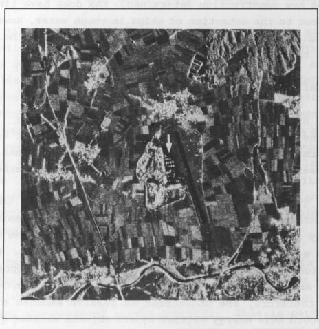
This SAR image was acquired over an airfield from an altitude of 10,000 m above the ground. Note the aircraft on the apron and their relative position near the runway. The length of runways and airstrips can be readily measured using this type of airborne imagery. (Image courtesy Intera Technologies Ltd.)
