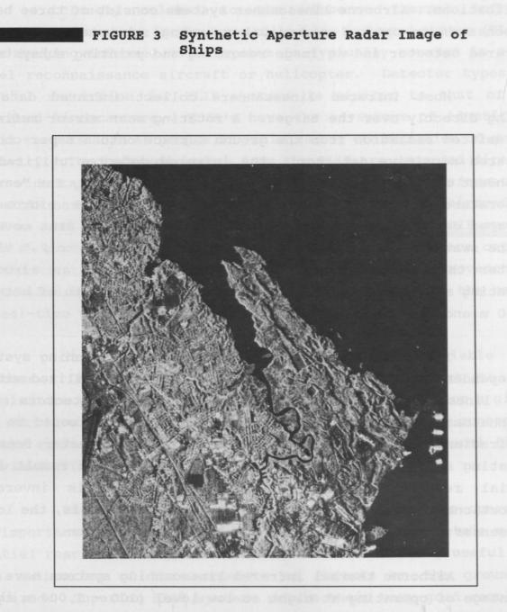
The bright targets on the right side of this SAR image are "mothballed" ships docked in a bay. Note the very high reflective signature exhibited by the ships. An airport is also visible on the image. (Image courtesy of Intera Technologies Ltd.) applications. Airborne linescanner systems consist of three basic components: an optical-mechanical scanning subsystem, a thermal infrared detector and an image recording and printing subsystem.
