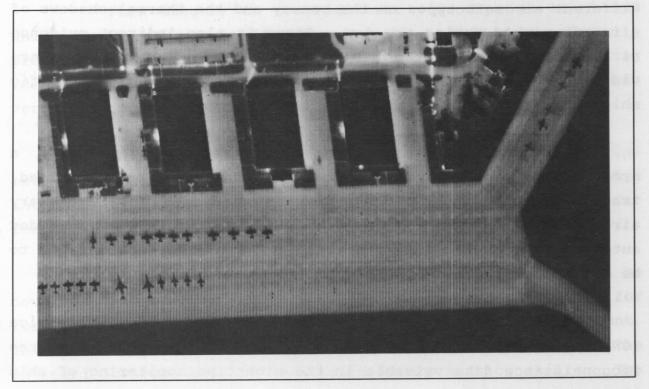
This thermal infrared linescanner image was acquired at night over a military air base. Note the different aircraft types and the thermal shadows of the aircraft parking areas during the previous day. Indirect evidence of human presence can be interpreted since the buried heating distribution lines are activated. (Images courtesy of the Canadian Department of National Defence)
