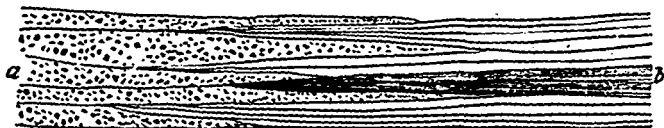
Diagram to show the “thinning out” of beds. a. Sandstones and Conglomerates. b. Limestones.
