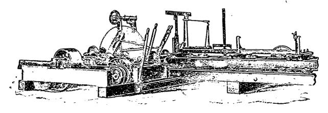
I make these mills with any number of Head-blocks spaced any distance apart. Equipped with Frost-dog, Knight dog, or Boss dog, Rope feed, or Rack and Pinion feed. With or without Over Log Saw Guide.
