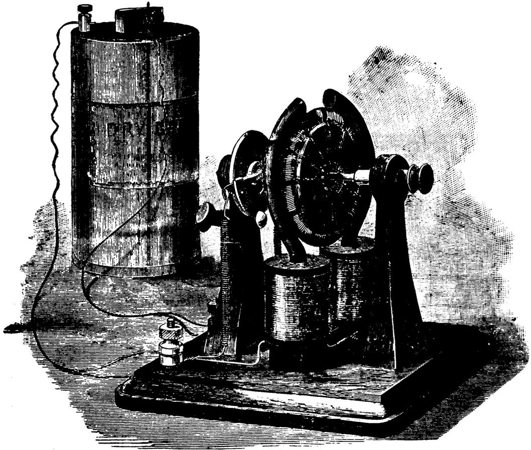
FIG. 1.—PERSPECTIVE VIEW OF A SMALL GRAMME RING MOTOR.
