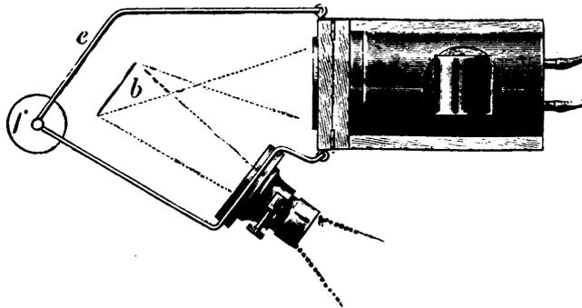
FIG. 5.—MEGASCOPE ATTACHMENT TO LANTERN.
