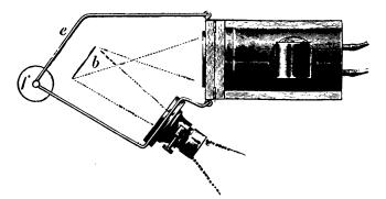
FIG. 5.—MEGASCOPE ATTACHMENT TO LANTERN.
