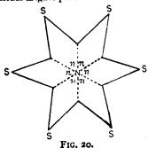
The six-nointed star shown in Fig. 20, is an anomalous magnet with apparently seven poles. The formation of the central N pole, as is evident from an inspection of the drawing, is due to the six separate morth poles, n, n, n, n, n, n, of the six separate magnets, Sn, Sn, etc. Such a magnet would be formed by touching the star at the point N with the S pole of a sufficiently powerful magnet.
