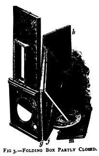
The length of the box inclosing the object and the burners is determined by the focal length of the object glass. In the instrument illustrated, the lens has a focal length of 24
