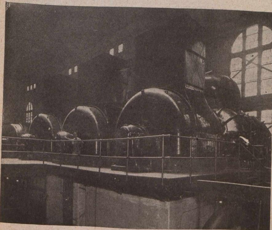
60,000 K.W. TRIPLE COMPOUND UNIT FURNISHING POWER FOR SUBWAY, SURFACE AND ELEVATED RAILWAYS OF NEW YORK—70,000 K.W. CAPACITY FOR TWO HOURS
