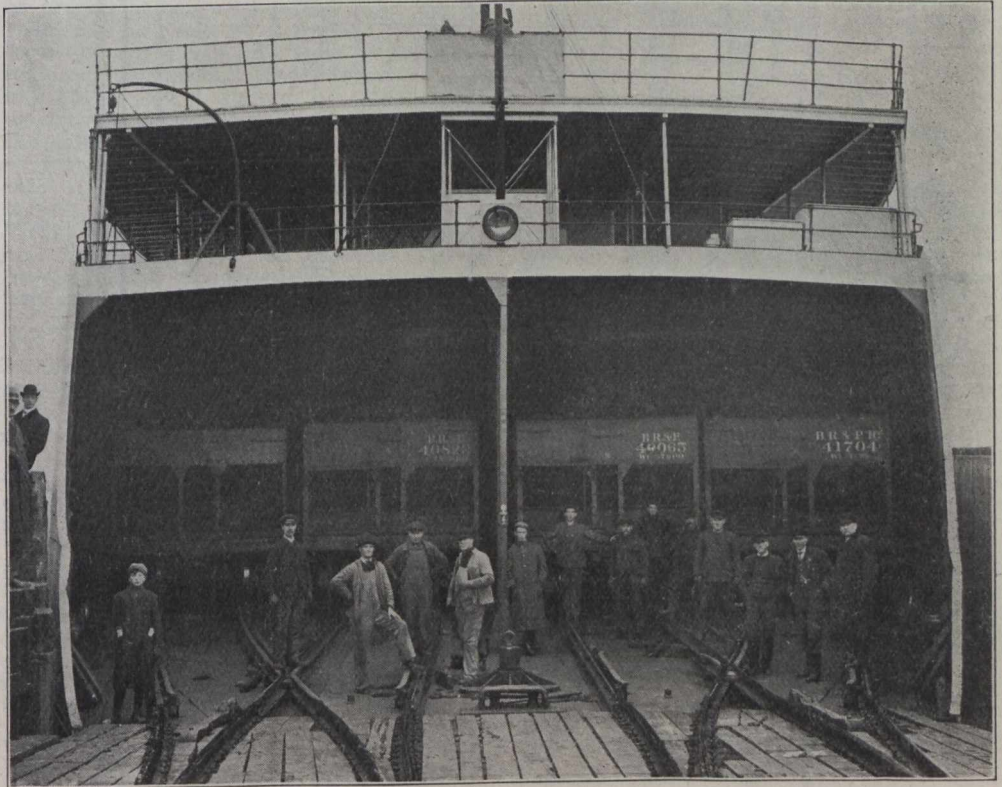
Stern View of Car Deck, Exactly the Same on Both Car Ferries.
