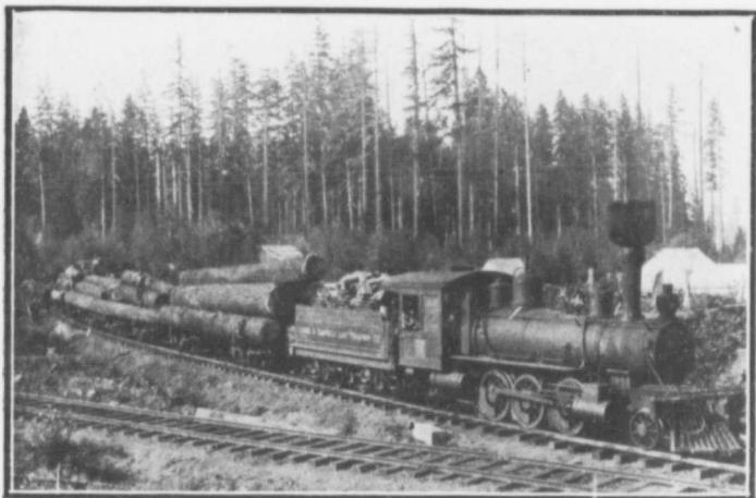
Getting out British Columbia's "wood crop." Rails are laid right into the limits. Note the screen on the smokestack to stop sparks flying.
