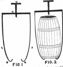
blacksmith can make. It is made to straddle the centre of the barrel, the legs (a, a) being light enough to spring a little when being placed in position, so that the toes (b, b) will clasp tightly the bottom chimes. The screw (c) passes through the centre of the top (d), which is made a little heavier in the centre on account of the
