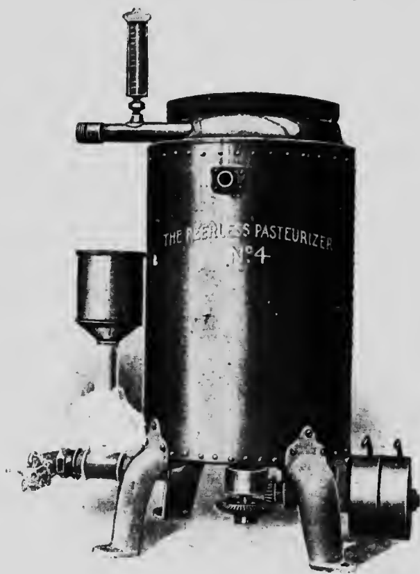
TYPE OF CONTINUOUS MILK OR CREAM PASTEURIZER.
