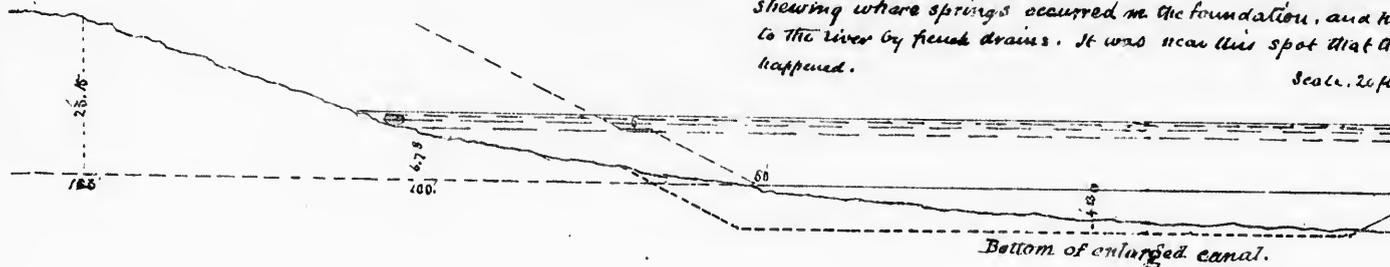
N<sup>o</sup> 4. Cross-Section of the canal on Sec. 11- upper reach, at Sta. showing section of the retaining wall built to protect the bank. This wall was entirely covered, out of sight, by the canal from the canal.
