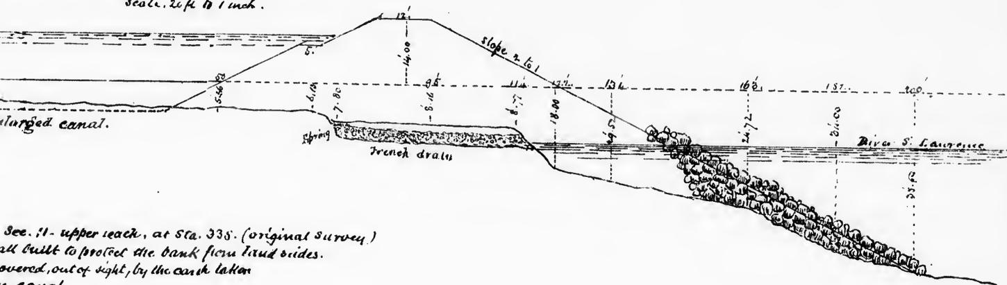
Sec. 11 - upper reach, at Sta. 338. (original survey) all built to protect the bank from land slides. covered, out of sight, by the earth taken from the canal.
