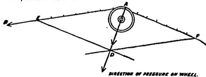
Set out AB and AC representing the angle made by the rope. Mark off AE and AF to any scale, say 1-in.=1 ton, representing the pull on the rope. Draw FD parallel to AE, and ED parallel to AF: then AD represents to the same scale the pressure on pulley (add to this the weight of wheel itself, when spindle is horizontal).
