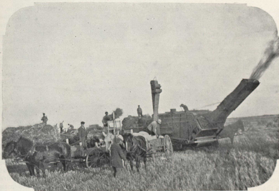
SHOWING THE HIGH-BAGGER, AN AUTOMATIC DEVICE WHICH ELEVATES THE GRAIN, WEIGHS A BUSHEL AT A TIME, AND DROPS IT DOWN THE CHUTE INTO A BAG HELD BY A MAN IN THE WAGGON
