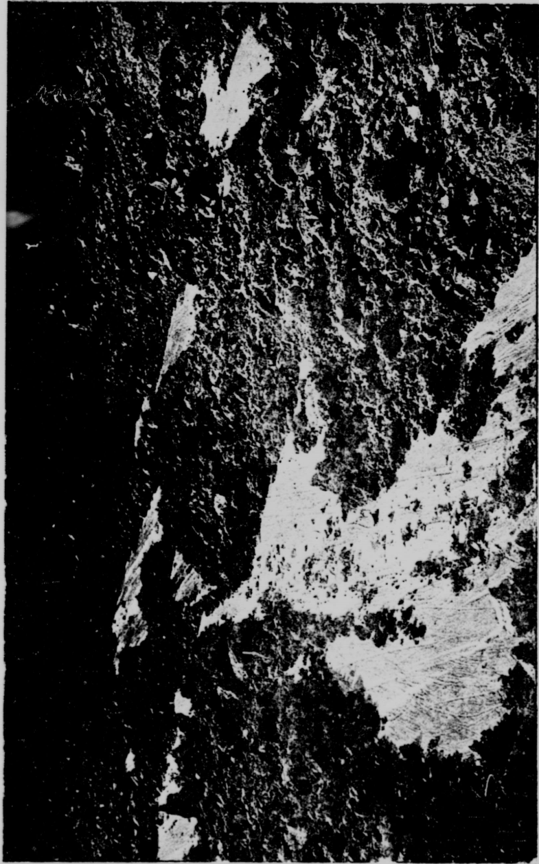
The gliding plane of clay striated by the gravel contained in the bottom of the moving mass of supersaturated clay.
