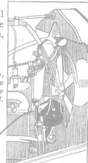
The indicator shows how the Northern Elevator and Timer looks when installed
