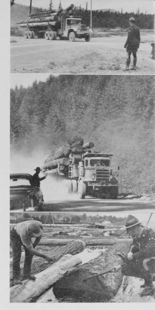
Top—This truck, on a private logging road is crossing B.C. Provincial Highway No. 1 on Vancouver Island. Note loose log on top and single safety chain. A few minutes after this picture was taken the top part of the load spilled onto the road.
