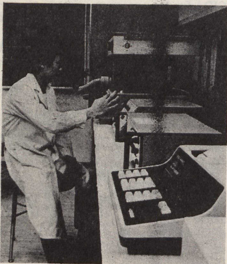
Graduate student Chung-Shun Ho operates a spectrofluorometer. A new process which he helped develop cuts bile acid testing down from several hours to as little as five seconds.
