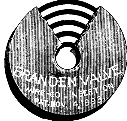
THE FIGURE REPRESENTS THE BRANDEN VALVE. PART OF THE RUBBER IS REMOVED TO SHOW THE WIRE COIL.
