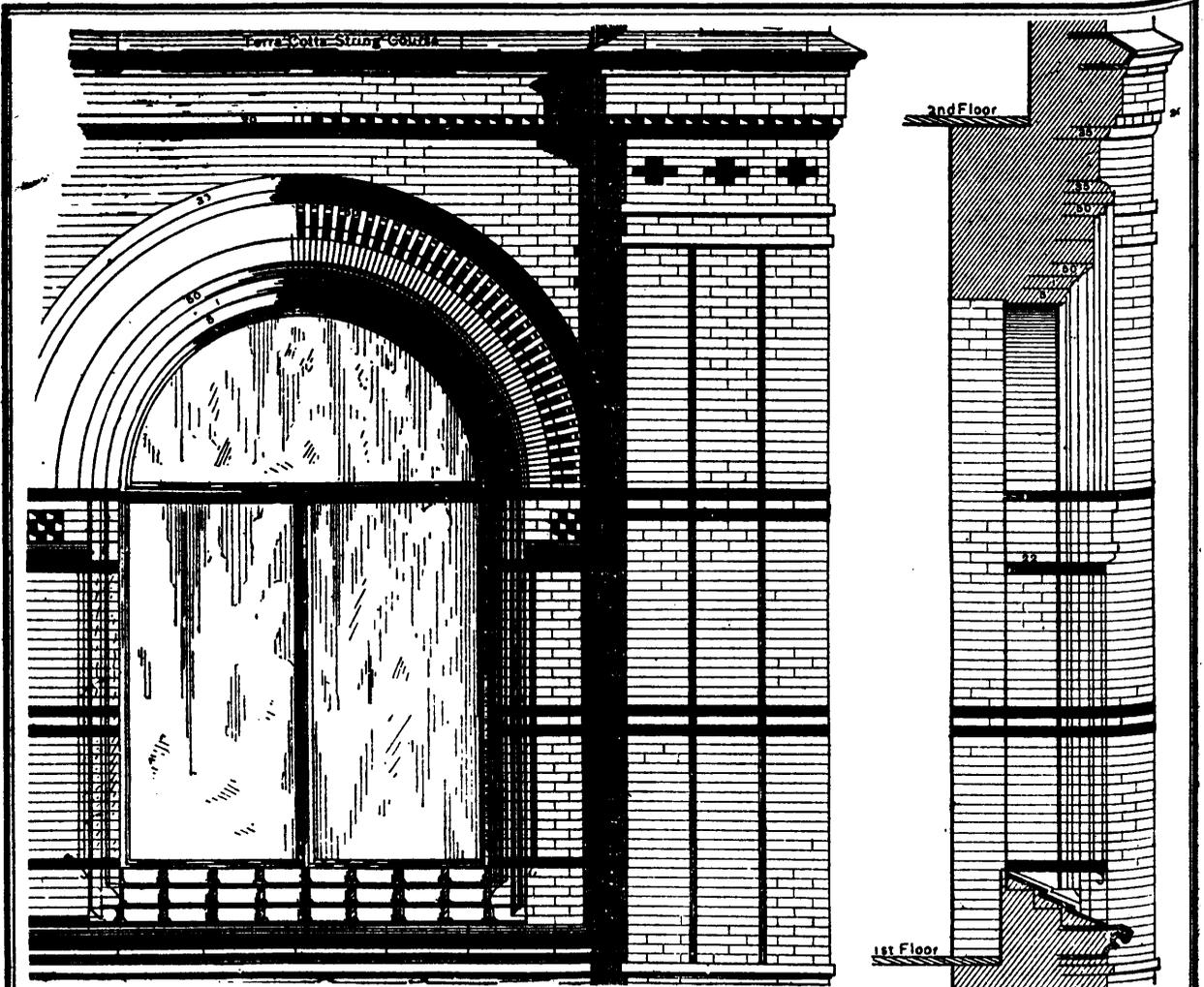
Artistic Brickwork.—Fig. 15.—Detail of First Story Windows of the New Morse Building.—Scale  $\frac{1}{4}$  Inch to the Foot.
