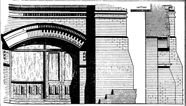
Artistic Brickwork.-Fig. 10.-Detail of the Basement Story of the New Morse Building.-Scale 1 Inch to the Foot.
