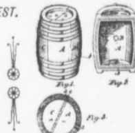
FIG. 1 is an exterior view of Cask. FIG. 2 is an interior perspective view of one section of the Cask. FIG. 3 is a transverse horizontal section through middle of Cask.
